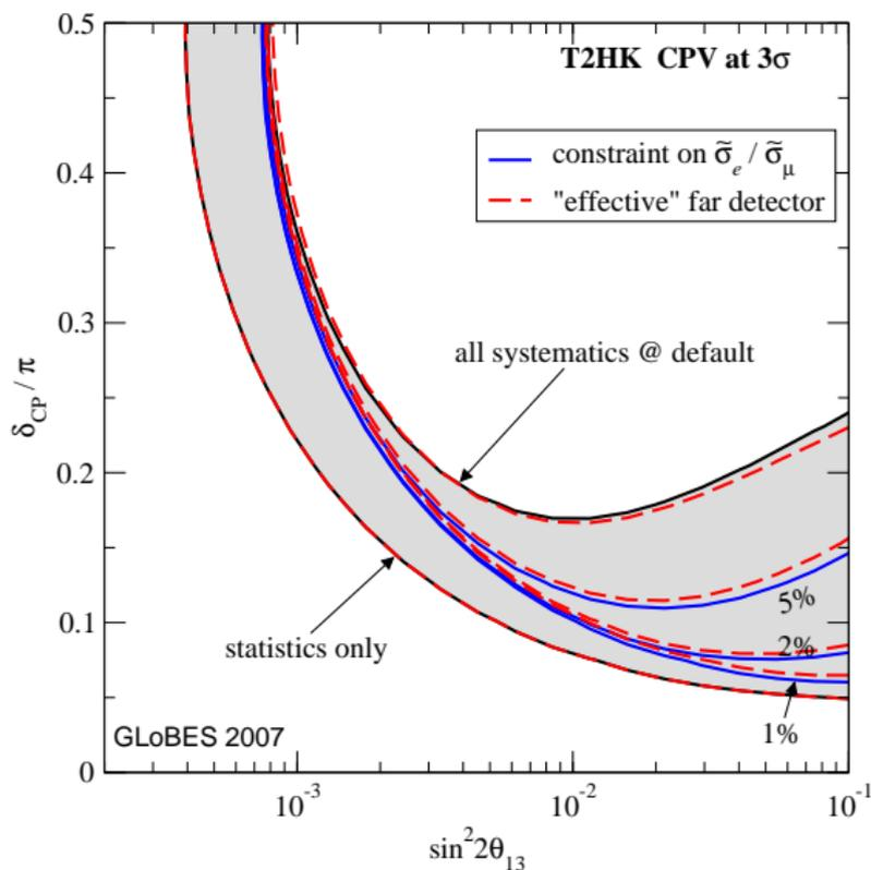
The 2 km close detector implementation is equivalent to overall systematic errors of 10% on signal and 3.5% on backgrounds.
