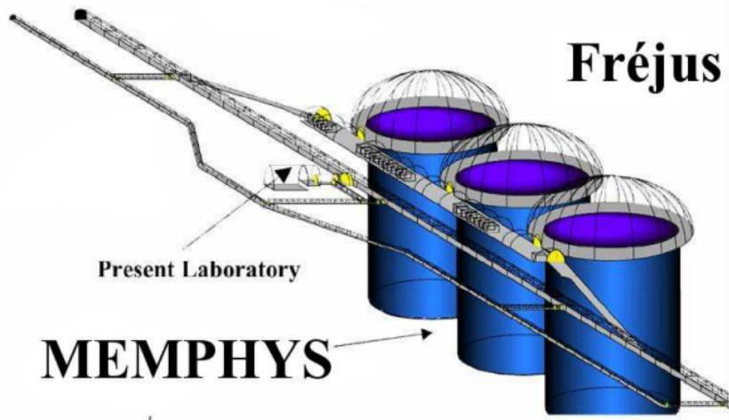
In the middle of the Fréjus tunnel at a depth of 4800 m.w.e a preliminary investigation shows the feasibility to excavate up to five shafts of about 250,000 m<sup>3</sup> each ( $\Phi = 65$  m, full height=80 m).
