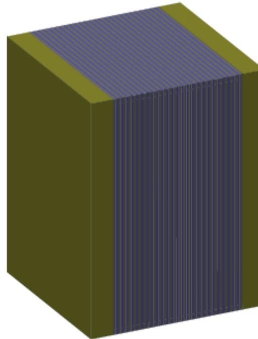
Figure 6.7: The POD detector viewed from the upstream end. The central region of the POD is constructed of alternating water target and scintillator tracking layers. The upstream and downstream regions are composed of lead radiator and scintillator tracking layers.
