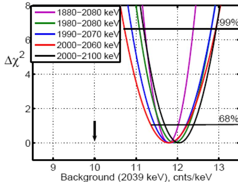
Figure 4.8:  $\chi^2$  as a function of the scaled model background for the five energy windows (Eq. 4.3). The arrow shows the background value obtained with an unconstrained fit (Fig. 3.13) in the 2000-2060 keV energy interval.
