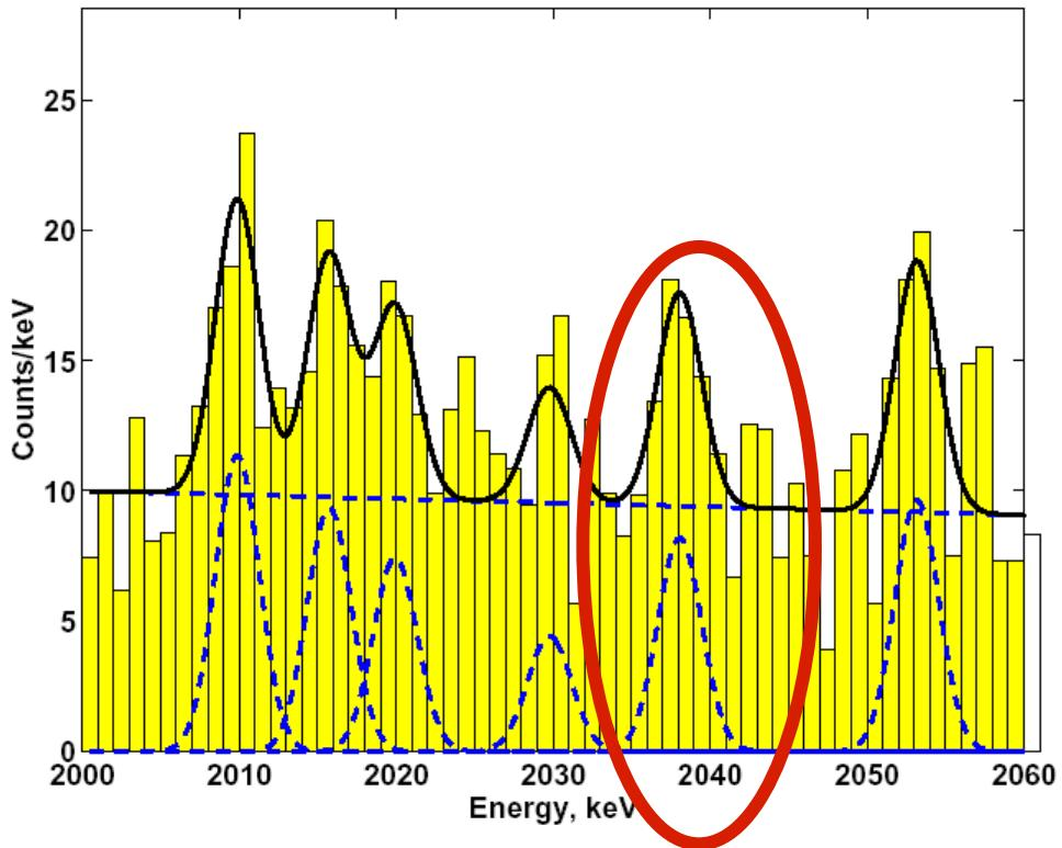
Fig. 17. The total sum spectrum of all five detectors (in total 10.96 kg enriched in  $^{76}\text{Ge}$ ), for the period November 1990–May 2003 (71.7 kg year) in the range 2000–2060 keV and its fit (see Section 3.2).
